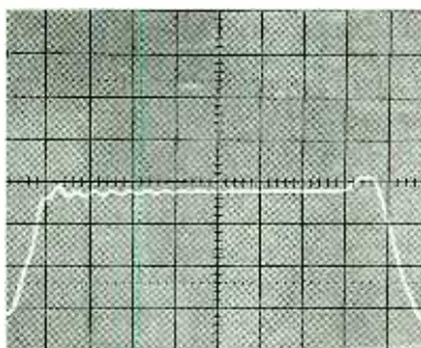
Fig. 6. Now we've shorted the far end of the cable. Instead of going higher, the reflected signal makes the display drop down. Not only does that tell us that the cable is shorted, it also can tell us the distance to the short.
