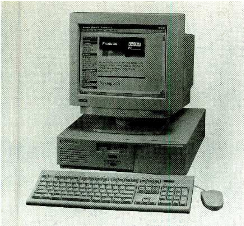
This DEC Venturis FX personal computer features a Pentium processor, EDO memory, and a pipeline-burst cache. It also features a "tool-less" case that is easier to open than traditional cases.
